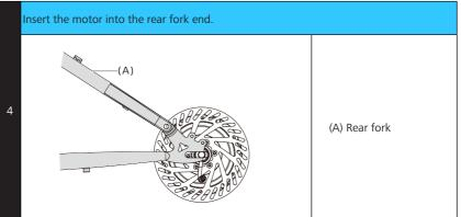
Place the stop pin onto the motor axle from the right side, then place the washers and cap nuts onto the motor axle respectively from both sides.
